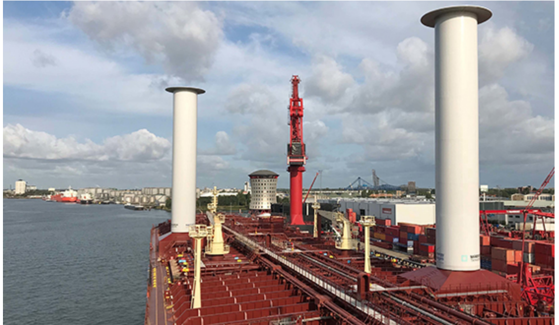
The Maersk Pelican oil tanker is testing Finland-based Norsepower's 98 foot deck-mounted spinning columns, which convert wind into thrust based on an idea first floated nearly a century ago. This photo shows the tanker Aug. 29 at Rotterdam, Netherlands. (Photo: Casper Hariot/Maersk Tankers via AP)
