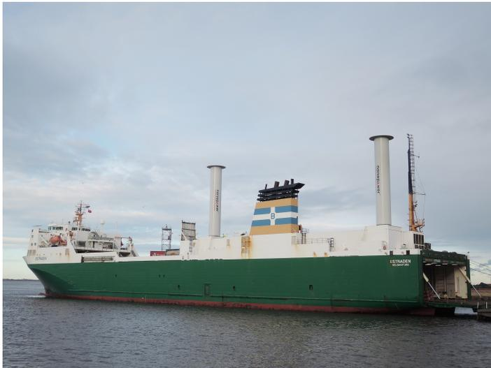
'MV Estraden' with the second Rotor Sail fitted. Photo: Norsepower
